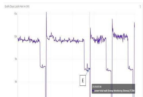
Figure-7. Heater power off
