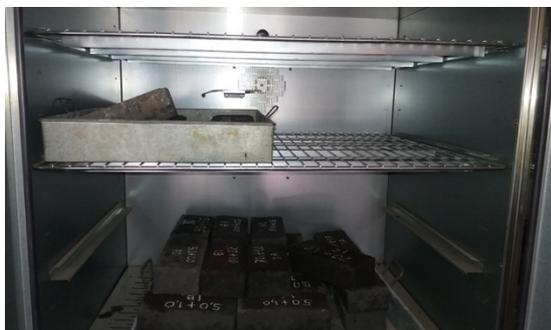
Gambar 4. Pengovenan *Paving Block*
