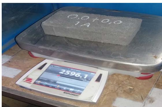
Gambar 6. Penimbangan *Paving Block*
