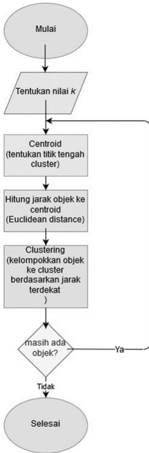
Gambar 2 Flowchart Algoritma K-Means
