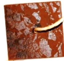
Figure 2 Specimen with chitosan inhibitor after soaking for one week
